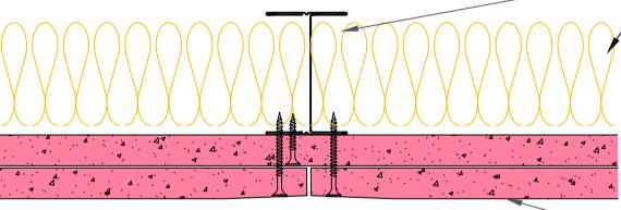
2x15mm Knauf Fire Panel fixed with SPEEDLINE Drywall Screws at 300mm centres (200mm centres at external angles). Ref to table for fixing length.
